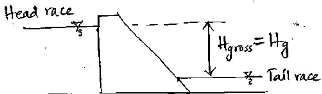
→ Difference b/w the elevation of Head race and Tail race is called "Gross head".
