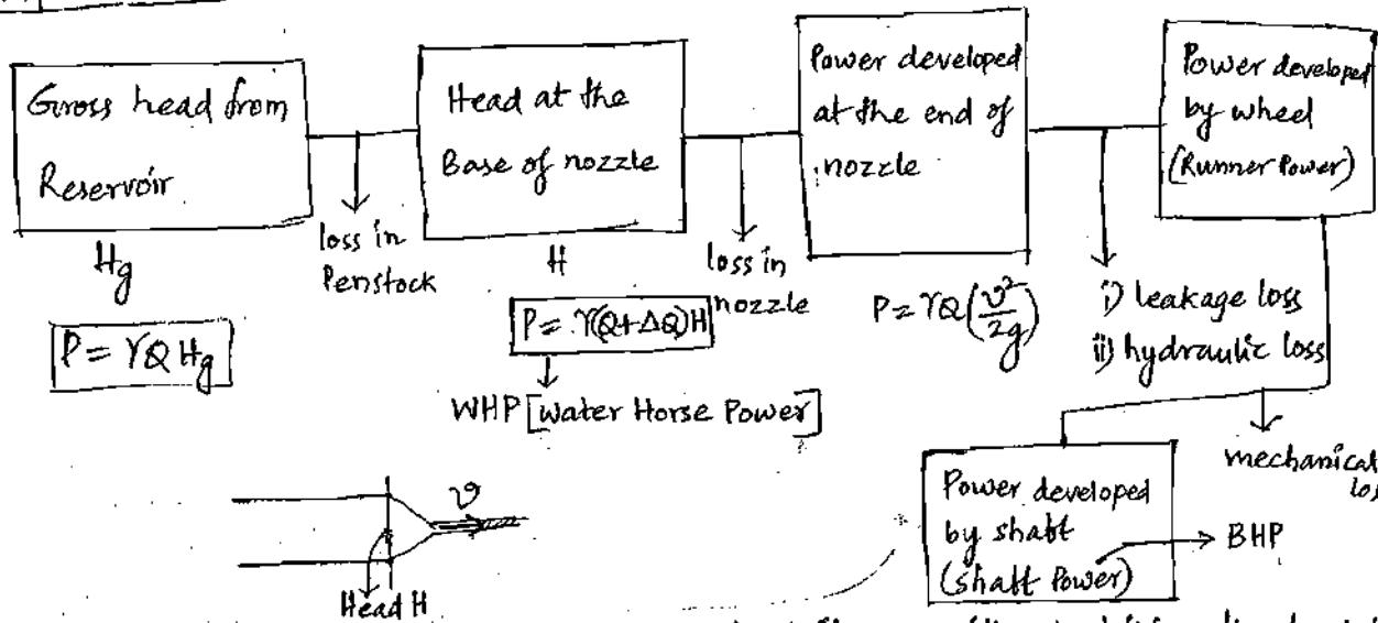
⇒ leakage loss → Accounts for water going to tail race without striking the buckets.
