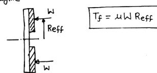
It is an imagamary radius for that we can assume the total friction force or the total Load is Acting
