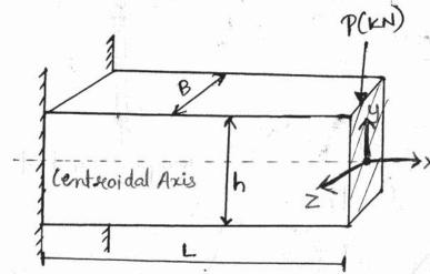
X→longitudnal Axis Y→ Teconsverse Axis Z→Lateral Axis
