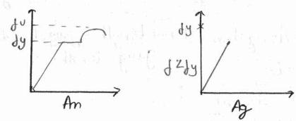
Note: -> Fau design of tension member connected with Rivet/80 lls there are two types of limit state
