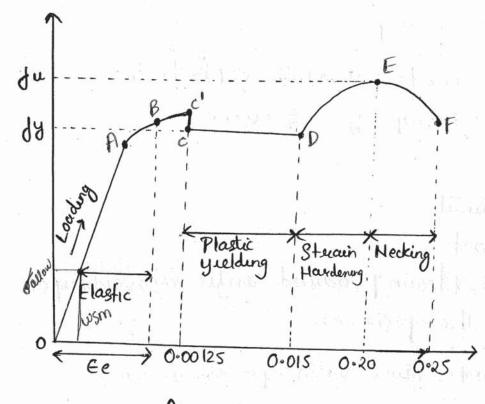
dy = yield steength (N/mm²) du = Ultumate tensile steength (N/mm²
