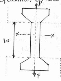
Ao→Orignal (ross sectional area (mm²) P→Applied load (KN)
