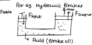
When Power is transmitted because of fluid Pressure.
