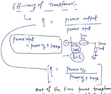
Most of the time power transformer operates on its rated Condition.
