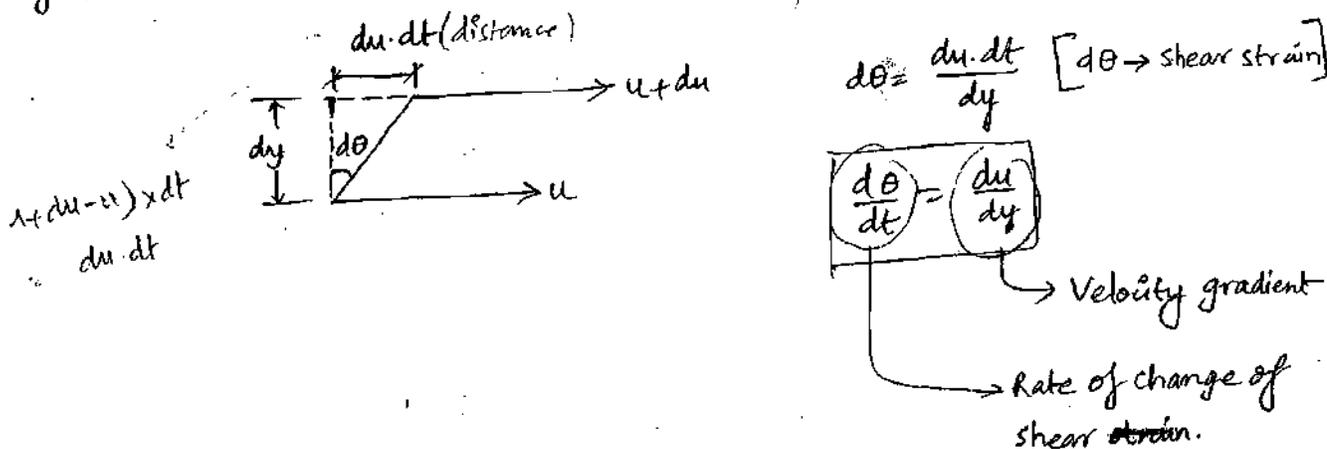
→ In case of Newtonian fluid, shear stress  $\propto$  rate of shear strain
