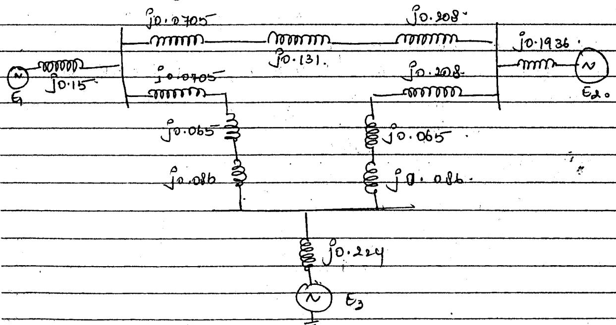
A 220 MVA, 66 KV, 3φ generator has  $x_{\text{sub}}^1 = 30\%$ , the 4 motors connected to 3 Motors through a Y-mission line and transformers as shown in fig, the motors have rated input of 60 MVA, 40 MVA, 100 MVA with 40%, sub-transient reactance, the rating of X-motors are shown in fig. draw the reactance diagrams assuming X-mission line reactance = 100%.
