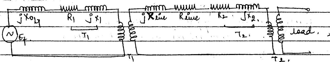
The eq. circuit of P.S. is complicated due to multiple component being present but single line diagram is a specified representation which is easily readable
