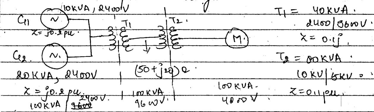
Choose base for Generator 1 as  $M = 25 \text{ KVA}, 4 \text{ KV}$
