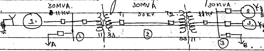
G<sub>1</sub> :- 30 MVA, 11 kV,  $X'' = 1.6 \Omega$ .
