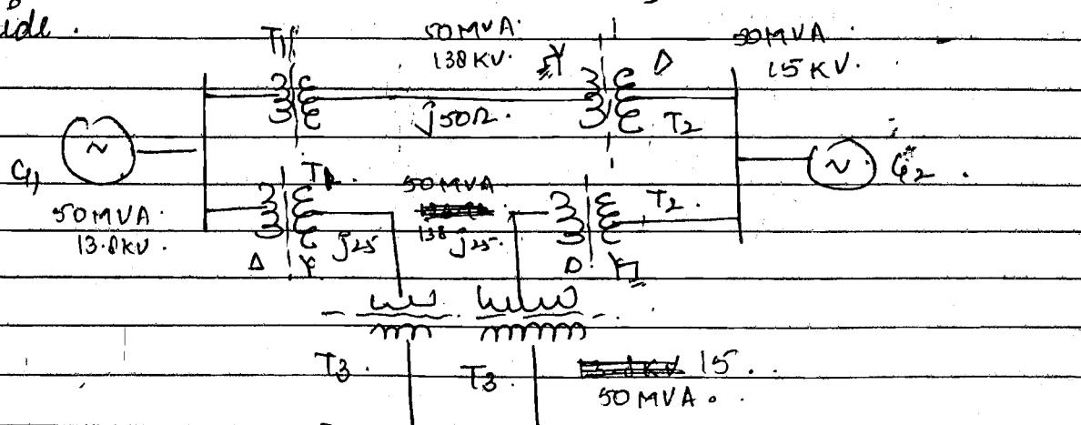
$$G_1 = 0.15 \times \left(\frac{50}{50}\right) \times \left(\frac{13.8}{13.8}\right)^2 \times 3002 = 0.15 \text{ p.u.}$$
