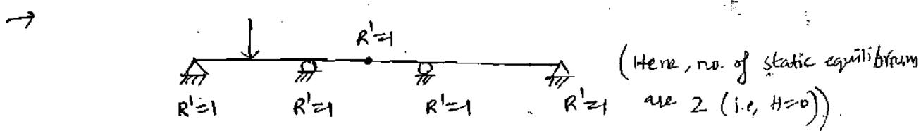
$$\begin{aligned} D_s &= 2C - R' \\ &= 2 \times 3 - 5 \end{aligned}$$
