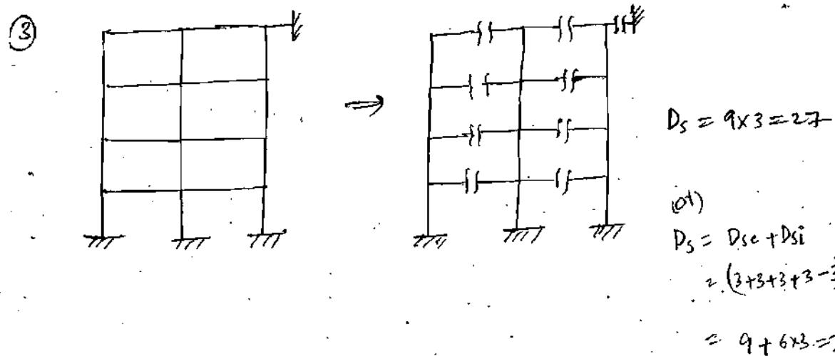
→ In case of frames ;  $D_s = 3C - R'$  → for 2D-structure
