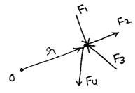
$$\Sigma \vec{F}_{0} = \vec{9}_{1} \times \vec{F}_{1} + \vec{9}_{1} \times \vec{F}_{2} + \vec{9}_{3} \times \vec{F}_{3} + \cdots$$
